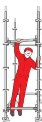
4. Insert 2 ledgers along the base of the scaffold, holding the standards upright allows these to be fitted at 90 degrees to the transom.
