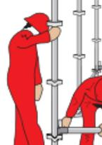
7. Now you can accurately position the tower to the structure and level the unit by using the adjustable jacks & a level. After you have levelled the base, tap the wedges in. This will make the scaffold firm.
