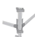
3. Place 2 standards on each of the first 2 jacks. One person should hold the 2 standards while the other person can fit the required transom to the standards. (Note: smaller standards nearest to main structure).
