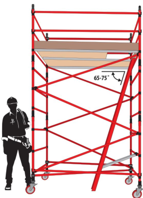
10. If the working height exceeds 3 times the least base dimension, the outriggers must be fitted.
