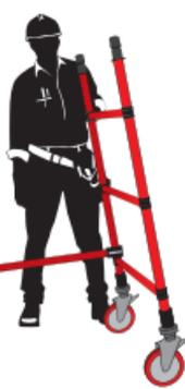
2. Attach horizontal brace (yellow brace) to vertical tube of base frame. Ensure castors are locked. Frame is now self supporting.
