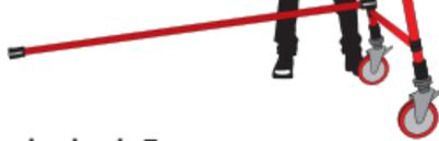
3. Attach spare end of brace to the other base frame. Attach 2nd yellow horizontal brace in similar position on the other side of base frames.
